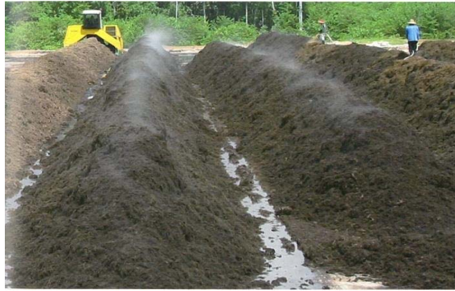
Figure 1.9 – An example of the “smoky” effect in a composting system in the open clamps of a triangular shape (source: https://tehnix.hr/en/ )
