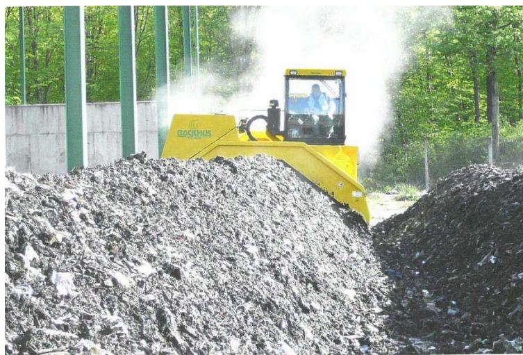
Figure 1.1 – The operation of the machine for turning over compost clamps (source: https://tehnix.hr/en/ )
