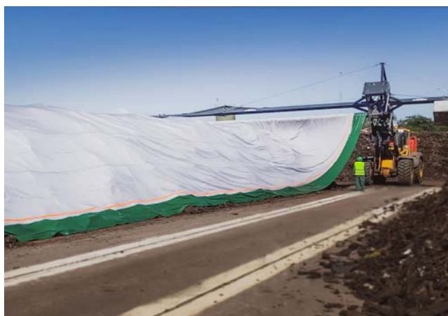
Figure 1.6 – An example of a membrane composting system (source: https://www.compost-systems.com/en/products )
