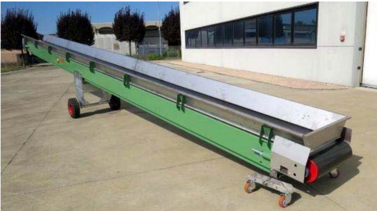
Figure 2.4 – Belt conveyor for compost
