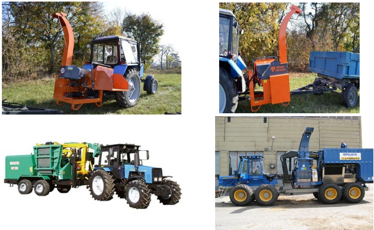
Fig. 5.2. Device for shredding green waste (tractor-based)
