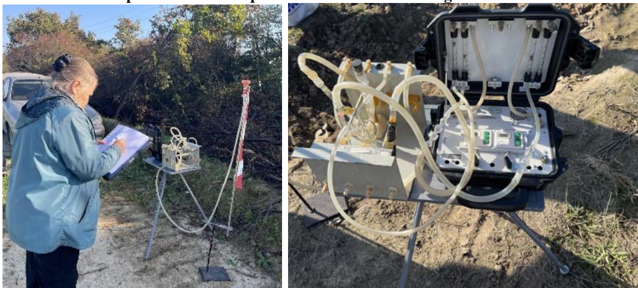
Fig. 3.14. Air sampling scheme for analyses the impact of the municipal waste landfill in the village Barvinok
